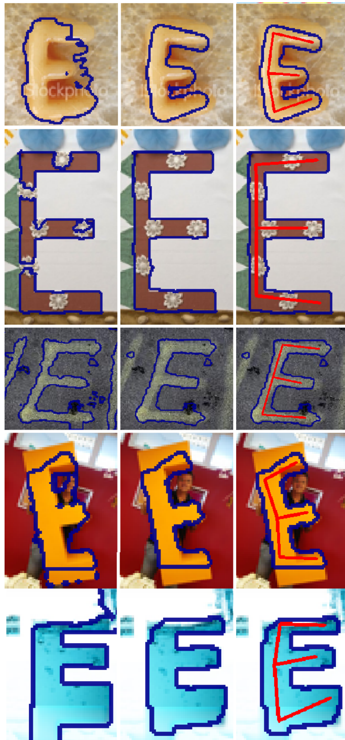
Fig. 9. Algorithm results for letter images. Left: segmentation without shape prior. Middle: segmentation with shape prior. Right: shape skeleton obtained during segmentation.
