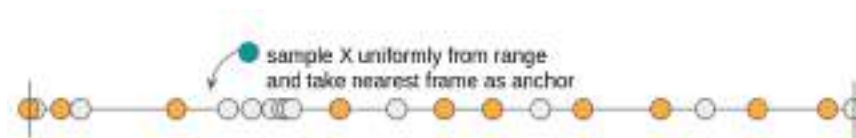
Рис. 4-1: Sampling from SYNTHIA dataset. Camera poses from two traverses (yellow and grey) are mapped to a line segment. Point X is sampled uniformly from the segment after which first image ( anchor ) is picked. In the neighbourhood of the anchor the same procedure is repeated to pick second image. This procedure ensures diversity of scenes and relative displacements in training set.
