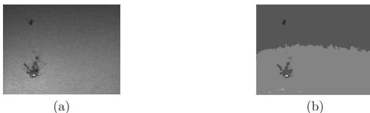
Fig. 1. Image of metal with foreign inclusions (a) before processing, (b) after processing.
